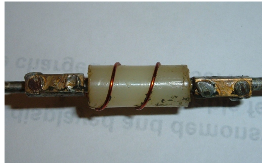
Close up of loading coil
