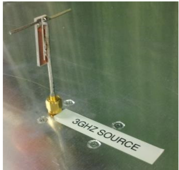
Halfwave dipole used as a transmitting antenna
