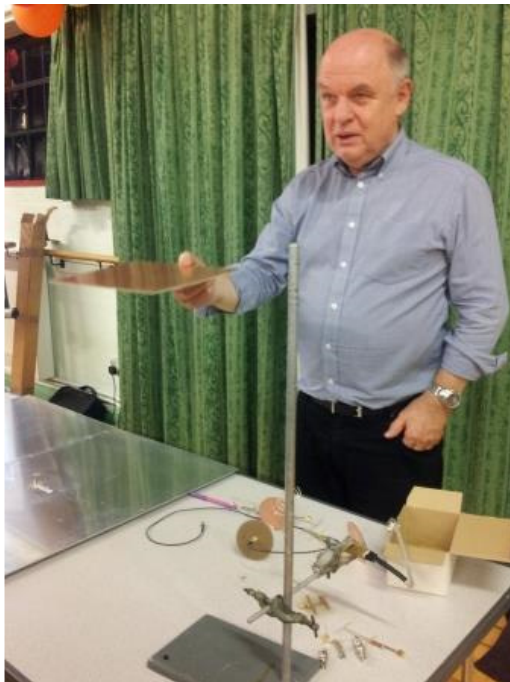
Terry raises and lowers his copper "ionosphere" to demonstrate the origin of HF QSB
