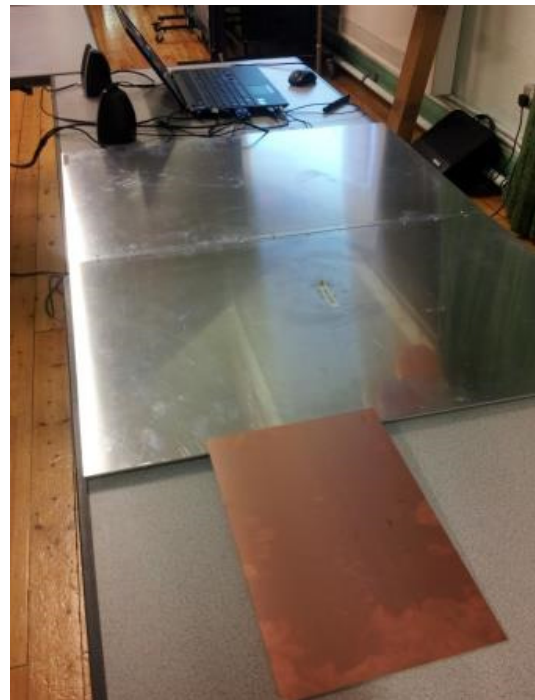
Terry's setup – folding aluminium groundplane with copper reflector "ionosphere" used later in the evening to demonstrate QSB (fading) effects
