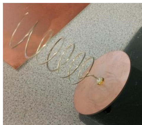
Helical antenna for 3 GHz
