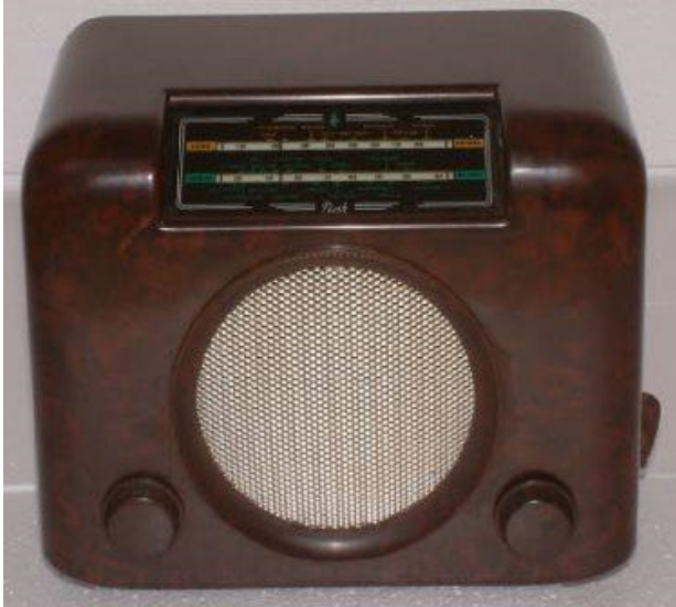
A Bush DAC90A similar to the one I used. Note the wavechange switch just visible on the right hand side of the cabinet.
